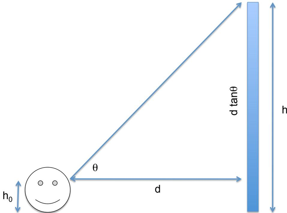
We will provide you with a measuring tape and an angle measuring device (clinometer). You are responsible for creating a useful data sheet. Record the height and radius of as many different trees as you can. To avoid duplication of data, coordinate with other groups
