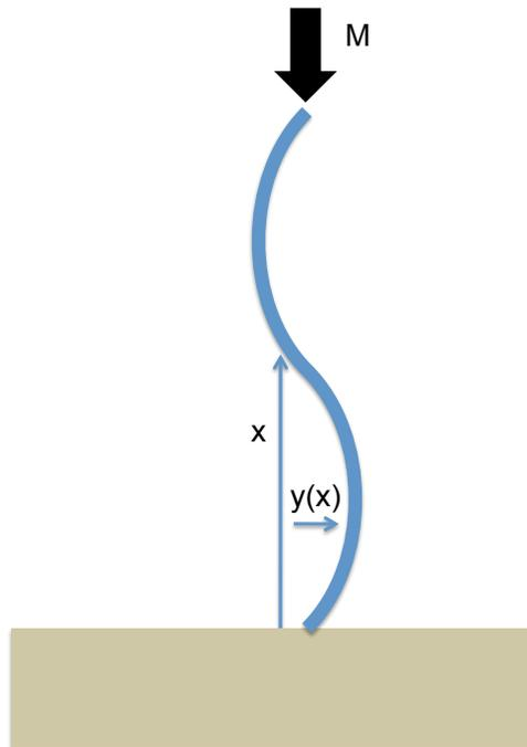
Now consider a column that has bent a distance  $y(x)$  perpendicular from the vertical
